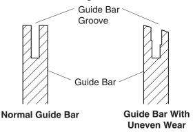
Figure 18 - Guide Bar Cross Section Showing
